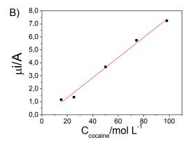
**Figure 5.** (A) Square wave voltammograms for successive additions of cocaine (in acetonitrile) to the electrochemical cell (frequency = 25 Hz and amplitude = 0.025 V) and (B) analytical curve for cocaine establishing the linear relation between the current and the cocaine concentration (in acetonitrile).
