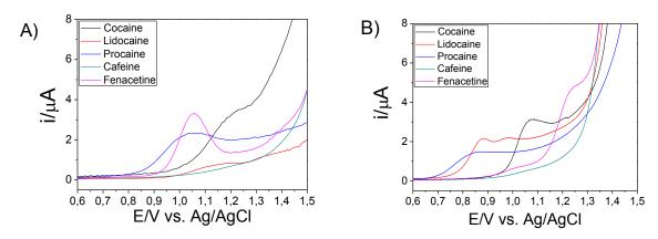
Figure 6. Square wave voltammograms of interfering substances (A) dissolved in acetonitrile (4.90·10<sup>-5</sup> mol·L<sup>-1</sup>) and (B) dissolved in acidic medium (9.96·10<sup>-6</sup> mol·L<sup>-1</sup>), both in the same conditions used for cocaine analysis.
