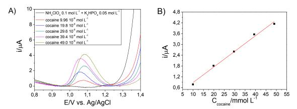
**Figure 4.** (A) Square wave voltammograms for successive additions of cocaine (acid medium) to the electrochemical cell (frequency = 30 Hz, amplitude = 0.06 V); (B) Analytical curve that establishes the linear relation between the current and the cocaine concentration (in acidic medium).
