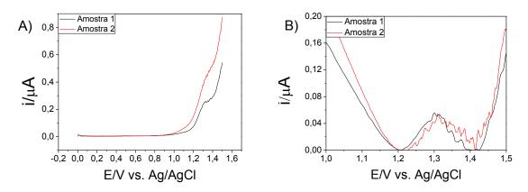
**Figure 7.** Square wave voltammograms of two seized samples of crack (A) dissolved in acetonitrile and (B) dissolved in acidic medium, in the developed method conditions.
