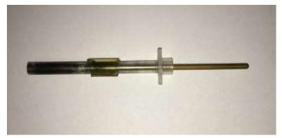
**Figure 2.** Carbon paste electrode after done.
