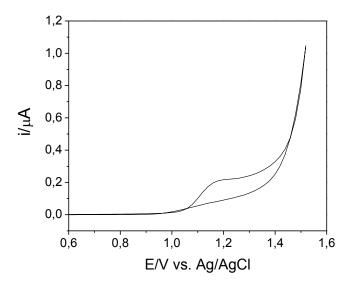
**Figure 3.** Cyclic voltammogram for 29.6  $\mu$ mol·L<sup>-1</sup> cocaine (acidic medium) in the electrochemical cell (v = 50 mV s<sup>-1</sup>).
