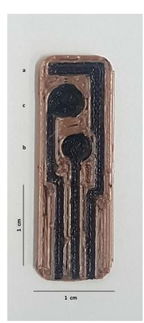
**Figure 1.** Three-dimensional printed electrode without the silver ink on the reference electrode; (a) counter electrode; (b) working electrode; (c) reference electrode.
